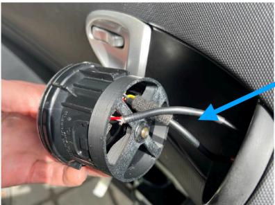
Connect the cables to the electronic board, passing through the bottom of the air vent.
