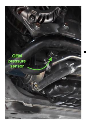
Remove the OEM pressure sensor
