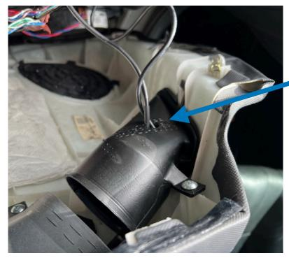
Make a hole in the pipe for the cables to pass through.
