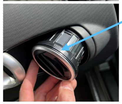
Replace the air vent, taking care to position it correctly.
